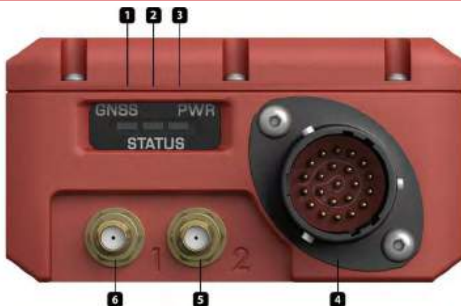
Figure 1. Connector panel of the RT1003
