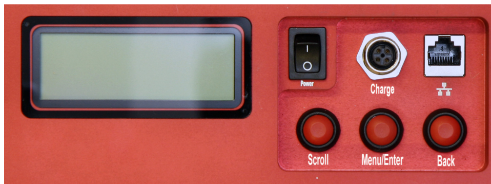
Figure 6. The control panel on the RT-Base S
