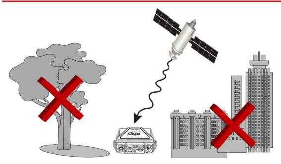
Choose a location for the GNSS antenna that is not close to buildings or trees, as these can both affect GNSS signals. The antenna needs to have a good view of the sky (not just above, but to the sides too).
