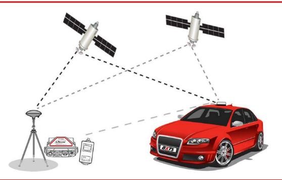
The base station is either placed at a precisely known location or left to average its position over time. It can then estimate the errors affecting each satellite it is tracking and broadcast information about those errors using radio modems. Nearby GNSS receivers use radio modems to listen for corrections, and apply them to the signals from the common satellites, reducing the errors in their own position calculations.
