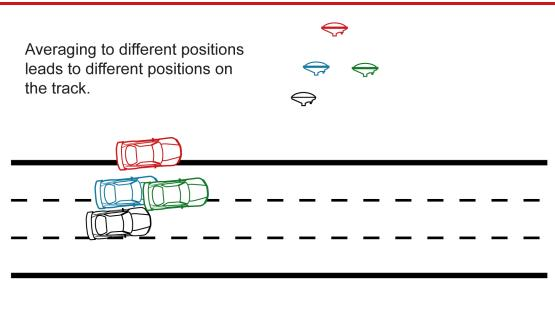
The problem of averaging to a different position happens each time that the GPS-Base goes through its averaging process. There is nothing magical about the GPS-Base that allows it to get its own position accurate to 2 cm or better. It is subject to the same errors that all GNSS receivers have and can only average its position to about 1.8 m CEP.
